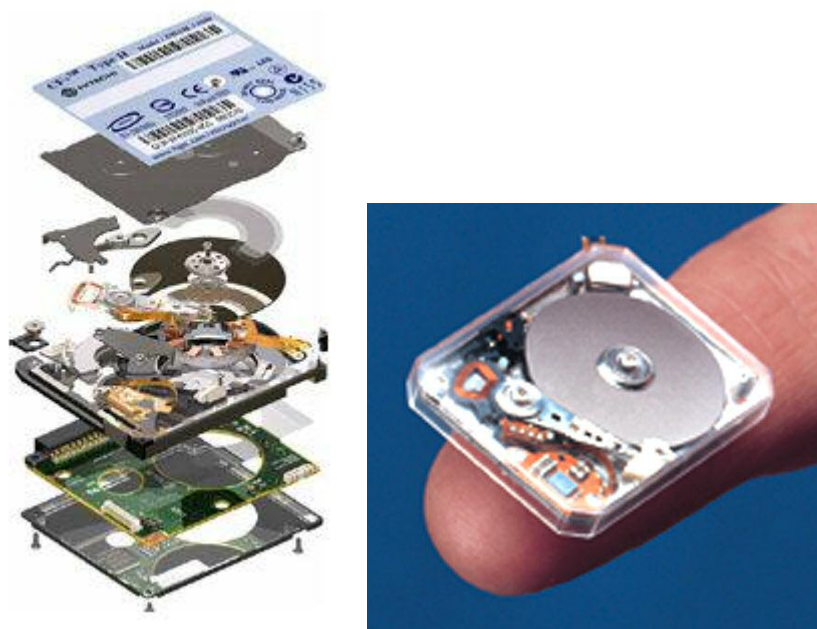
Figure 1.1 Toshiba's 0.85 in. HDD can store 4 GB of data ( February 2005 issue of Smartphone & Pocket PC ).
